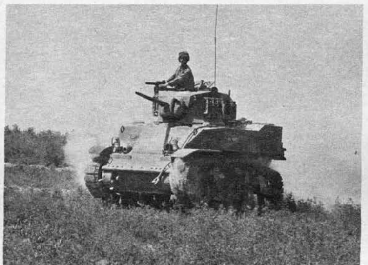
M-5A1 silhouette is high but tank is protected by slanting, welded armor. Typical U.S. suspension has two pairs of tandem bogies.
